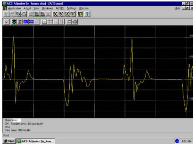
Fig. 7: Dynamic error position (y-axis: 50 counts per division).
