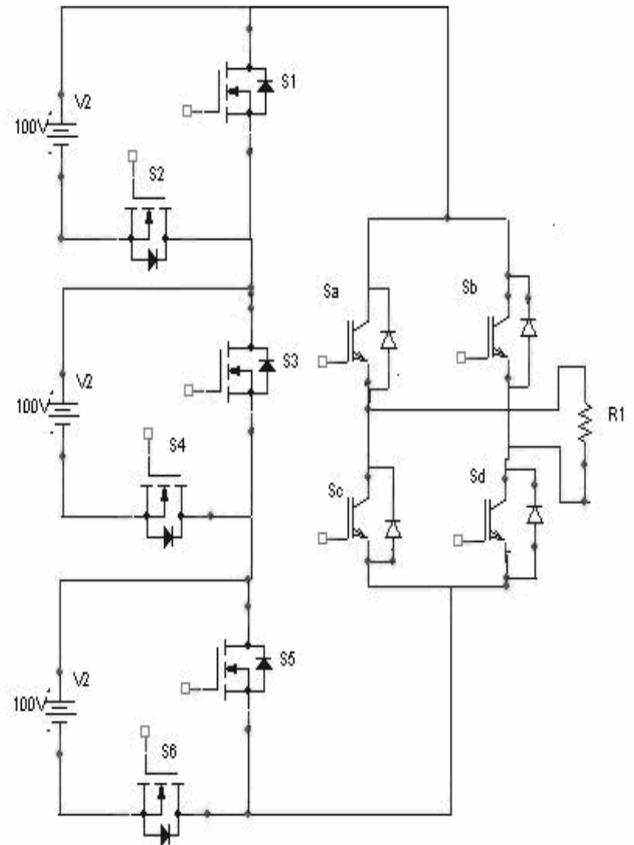
Fig. 2: 7-level Cascaded multilevel DC link inverter
