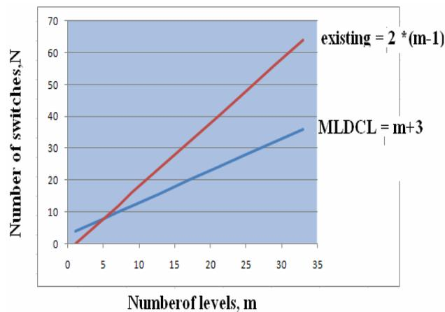
Fig. 6: Comparison of required number of switches.
