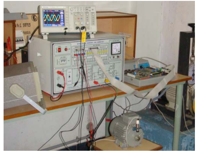
Fig. 9: Experimental setup of three-level inverter
