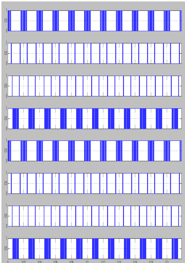
Fig. 10: Gate pulses for phase-A of five-level inverter
