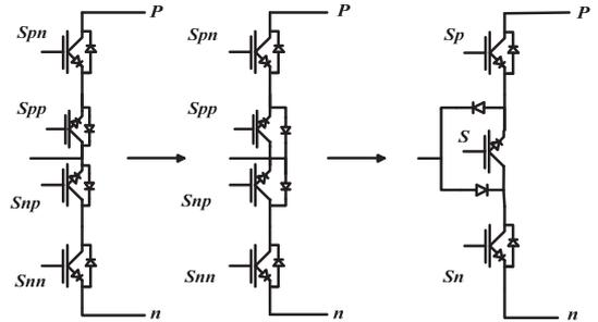
Fig. 3: Steps to reduce the switch number.
