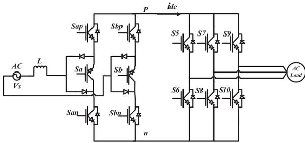
Fig. 4: A Reduction of switch number from 14 to 12.
