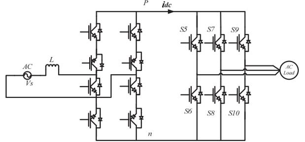
Fig. 2: Topology with 14 uni-directional voltage blocking switches.
